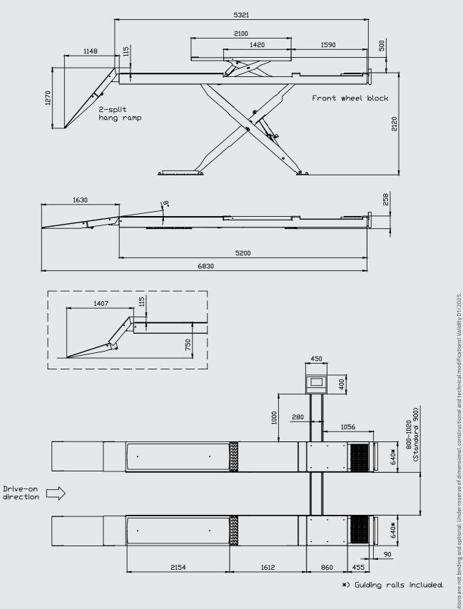
The MagiX 50-52 can also be installed recessed in the floor. You can find more information and dimensional sketches at www.autopstenhoj.com.
