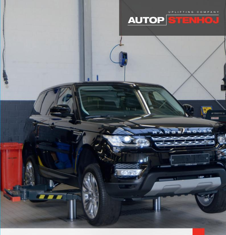
Electro-hydraulic twin-ram lift, 3.5 t with adjustable swivel arms
