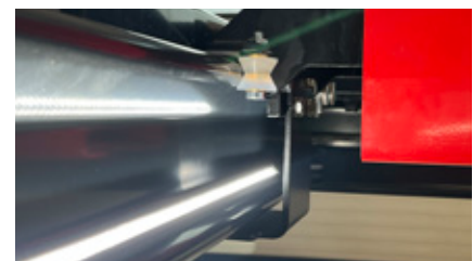
Roller suspensions for scissor jack on the inside of the platform profile
