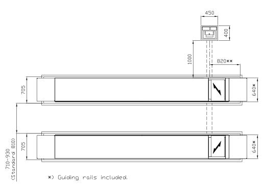
\*\*) Dimensions for recesses are for drive-through versions (4 x short ramps) for further options see foundation drawing T82336
