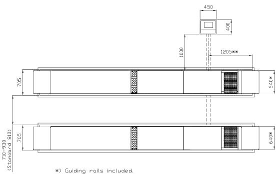
\*\*) Dimensions for recesses are for drive-through versions (4  $\times$  short ramps) for further options see foundation drawing T82337
