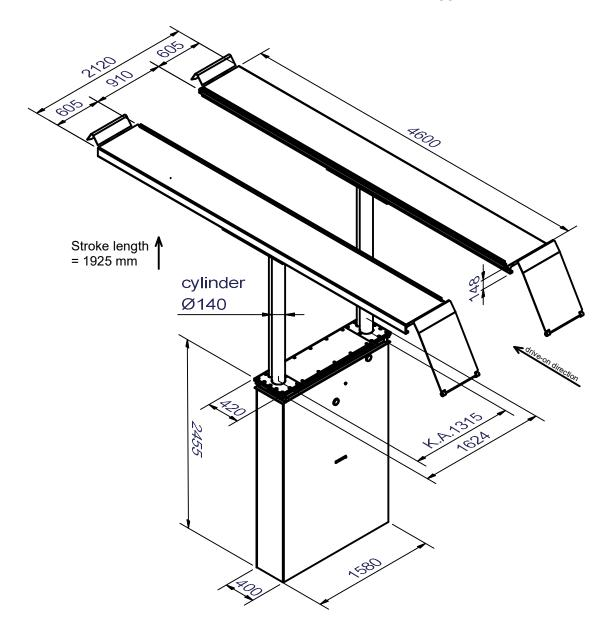
Dimension sketch incl. specifications of level for drive-over height.
