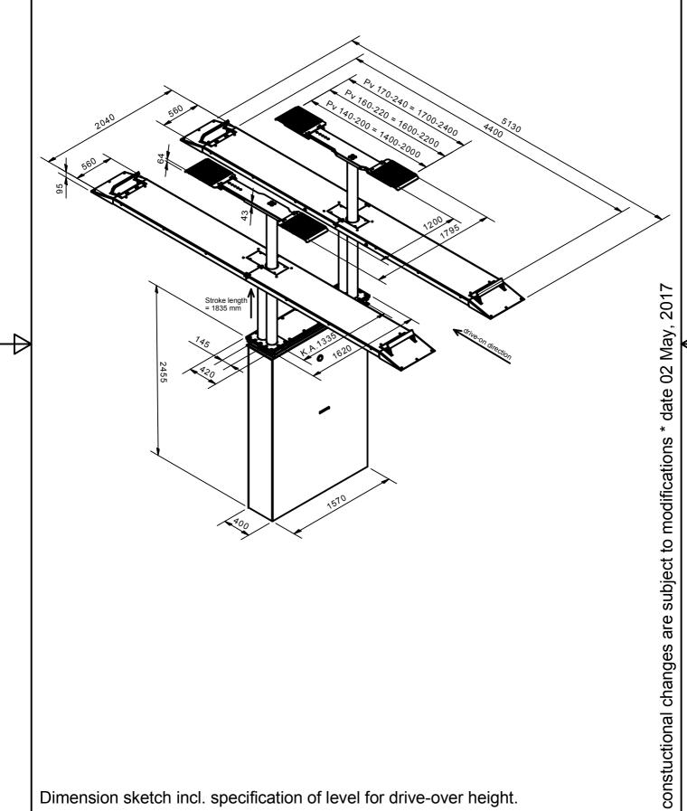
Dimension sketch incl. specification of level for drive-over height.
