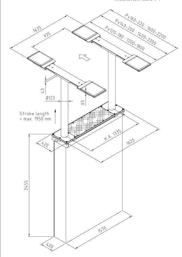
Dimension sketch incl. specification of level for drive-over height.
