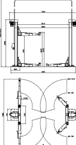
The 2-post lifts of the Maestro 2.xx series impress with their premium construction. They come with extremely stable and welded columns. Smooth running behaviour is ensured by the **roller-bearing carriage**. The cold-rolled spindle guarantees a particularly long service life. The welded and symmetrically installed posts are perfectly suited for lifting large and heavy vehicles up to 6.5 t at
